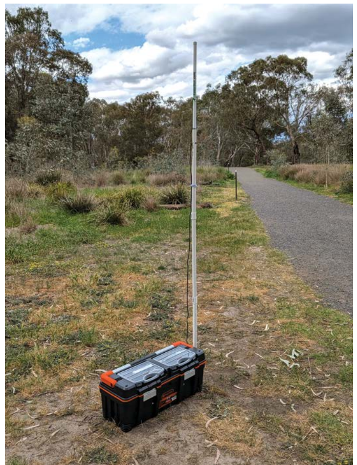
Low cost, portable, self-contained ADS-B field receiver – Image: FRV
